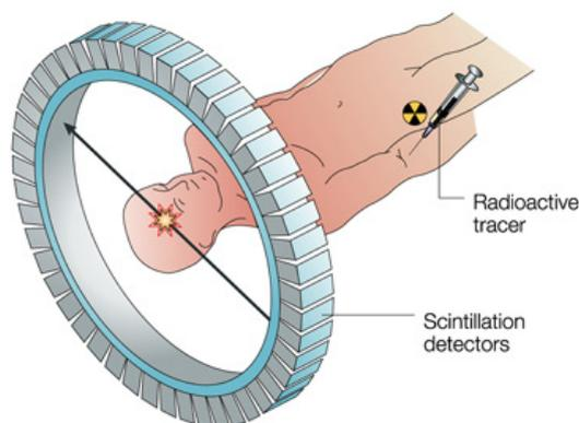
Fig. 1. A schematic illustration of a patient in a PET-scanner. Reprinted by permission from Macmillan Publishers Ltd: Nature Reviews Cancer, copyright 2004 [15].
